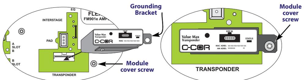
**Insert transponder with grounding bracket into transponder socket**
